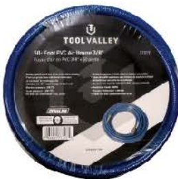
77319 - 3/8" x 50' PVC Air Hose Includes 1/4" npt male fittings at each end. Working pressure: 300 psi, burst pressure: 1200 psi.
