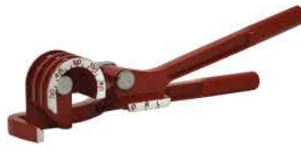
77314 - 180° Tubing Bender Makes short, smooth radius. Bends up to 180 degrees. Comes with a calibration gauge to indicate angle of bend for copper, aluminum and thin wall tubing. 3/8" max. bending capacity. For 1/4", 5/16", 3/8" o.d. tubing.
