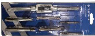
56231 - Metric Tap Set 8 pcs Includes: tap handle and 7 taps. Taps: M3x0.5, M4x0.7, M5x0.8, M6x1.0, M8x1.25, M10x1.5, M12x1.75.
